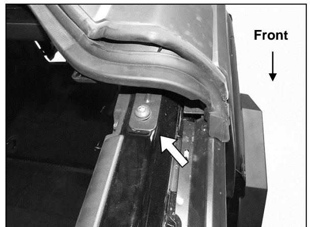
(Fig 20) Insert Top Roof Spacer between top bracket (arrow) and inner roll bar (driver/left side pictured)
